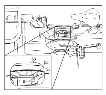
Next, rotate the Crank Pulley (53) until a Magnet (55) is aligned with the Reed Switch (35). Slide the Reed Switch slightly toward or away from the Magnet. Then, retighten the #8 x 19mm Tek Screws (97).
